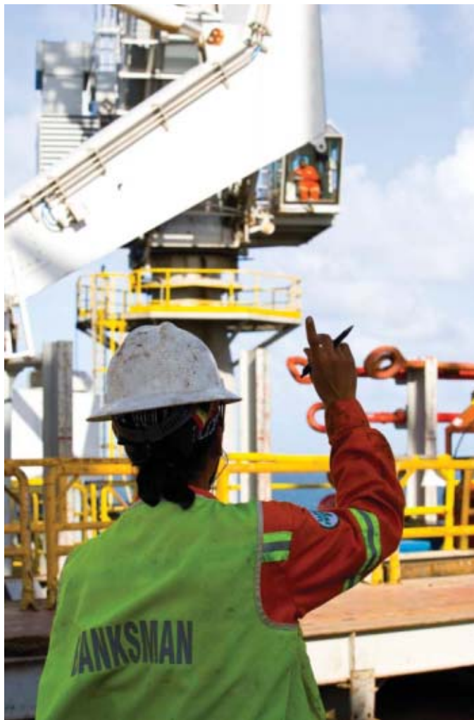
The banksman works with the crane operator to ensure that lifted items arrive safely. Photo from Transocean.
