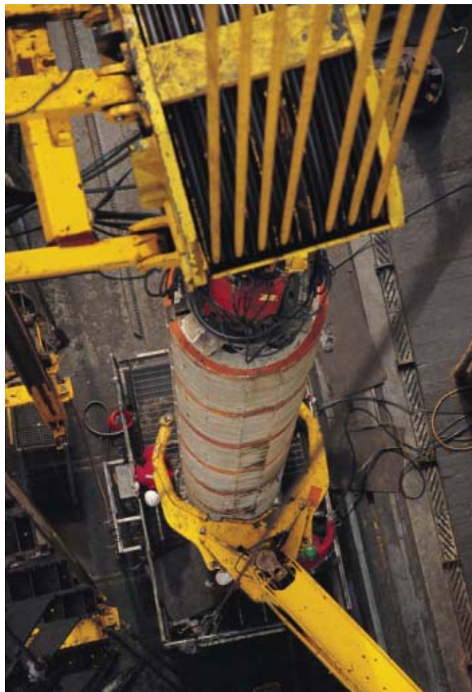
This riser-handling mechanism on the Transocean Deepwater Discovery ultra-deepwater drillship off West Africa is an example of the automated equipment that is helping to make offshore drilling safer and more efficient. Photo from Transocean.
